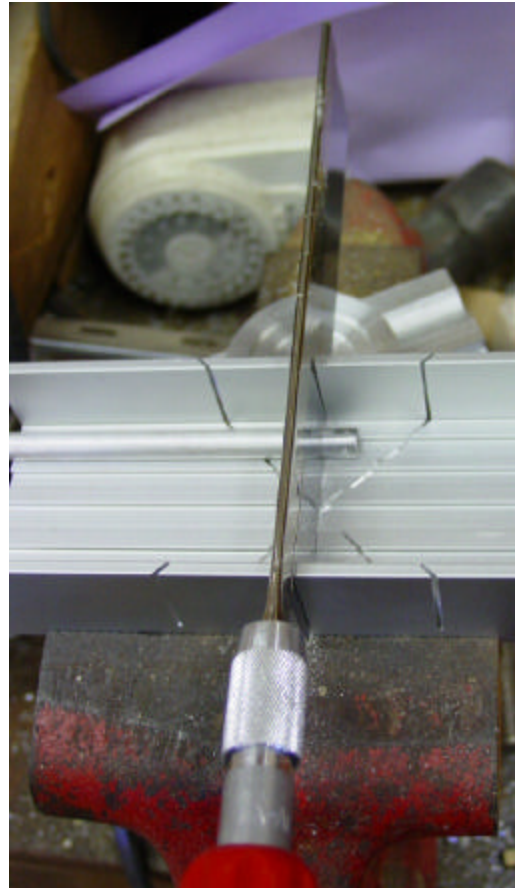
Use a razor saw and miter box to cut the tubes. Be sure to debur everything.
