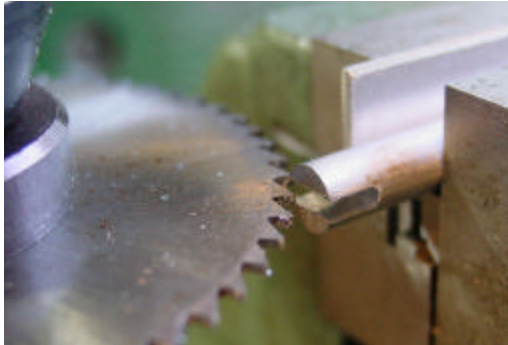
Cut the slot in the piston rod.
