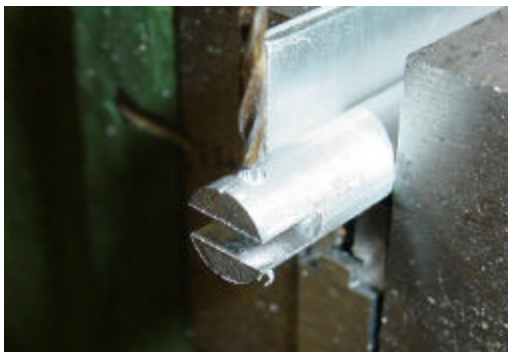
Cross drill the piston at 90 degrees. Do it all in one clamping if possible. Parts are small so center drill everything.
