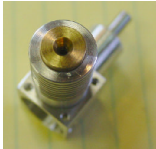
Valve seat is sealed to cylinder by snug fit and LocTite.
