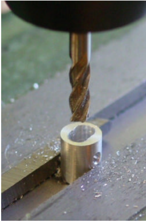
Mill inside of piston, keep 90° to pin hole.
