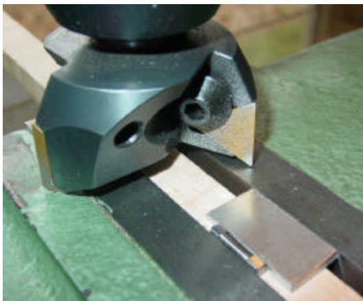
Mill flat sides on connecting rod.
