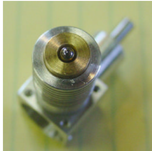
Ball in seat. The pin height should lift the ball about .015 at TDC.
