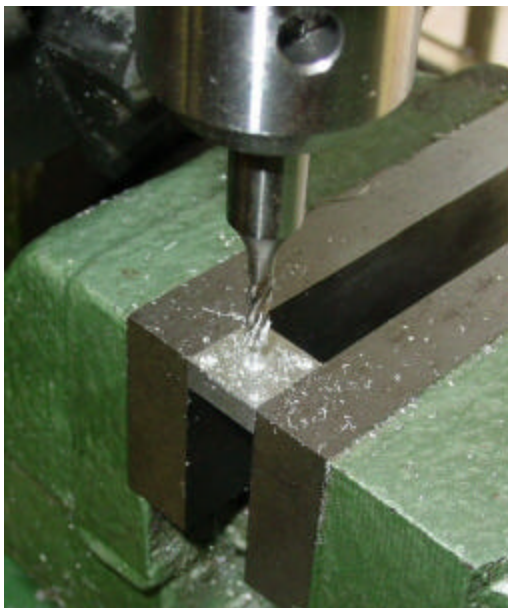
Use ball mill to make the socket for the valve ball.
