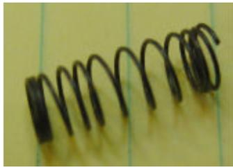
Three different compression springs are used in this engine. They are all the same size and number of turns but use different wire sizes for different strengths. Make the mandrel from a section of drill rod. Turn down the areas at the ends of the springs, cut a partial thread at the desired spring pitch to guide the wire.
