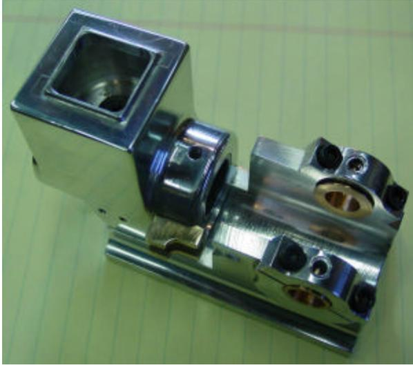
The Main bearing supports and cylinder are mounted to the base. Verify the sides are parallel to each other and parallel to the side of the cylinder. Ream the main bearings .001 larger than the crankshaft diameter. Do this in the milling machine so it will be square and true. Turn the reamer by hand so it does not make an oversize hole.
