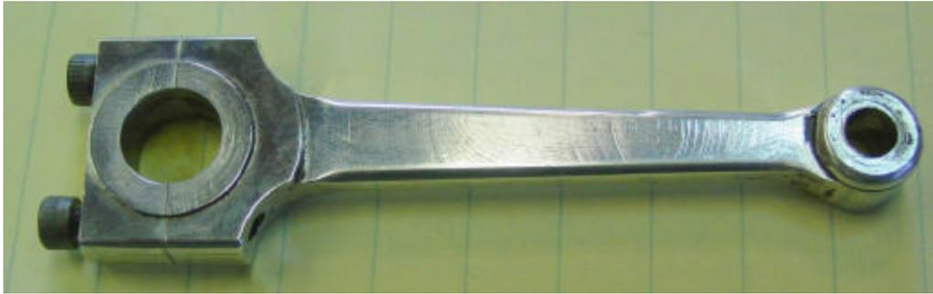
The drawings note that a brass or bronze bearings can be added. There is sufficient material to add these. The actual design is not critical. The Crankshaft above has no measurable wear and has been in service for 30 hours.
