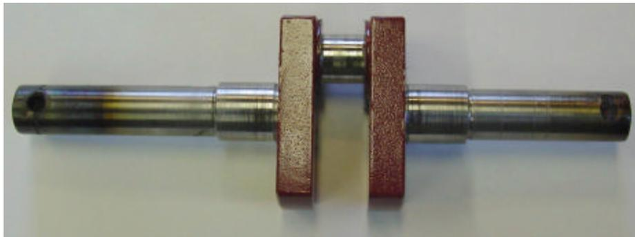
Start turning the crank pin. I used a parting tool to make the deep cuts. Slow feed and re-sharpening before the last cut produced a good finish.
