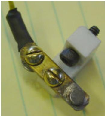
The other finger is made of ridged brass. It is mounted on a plastic insulator. This part of the points is the contact that triggers the ignition circuit.
