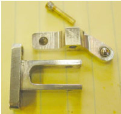
These parts are straightforward. A SS ball bearing is inserted into the rocker arm and should end up centered on the exhaust valve. The hardness of the ball and its shape will make the valve operate well. The arm needs to move about 10 degrees freely in the pivot.
