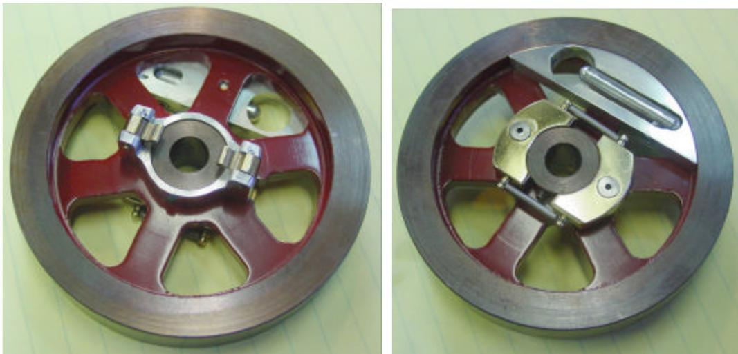
I added a spring loaded starting lever. It is not needed now that properly designed parts are used. In the beginning, hundreds of flips happened with no running. Now that all of that has been overcome it starts on the first flip and this is not needed. Add it if you want to.
