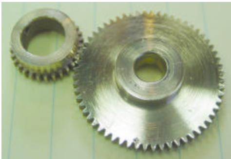
Make the gear blank and mount it on the rotary table on an arm to give the cutter clearance. The gears are all based on dull degree movements so they are easy. Make the first cut and measure to the first cut depth shown using a drill bit in the slot. Then just rotate and cut. It is fast and easy and you get a perfect gear.
