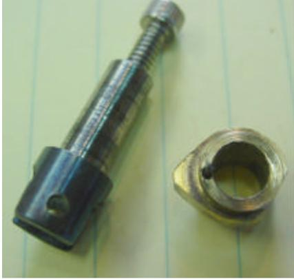
This cannot be cut until the engine is nearly complete and timing set. First cut the flat to about  $\frac{1}{2}$  the depth shown and assemble the engine and see where the points open. At this point it should be a few degrees before TDC. As the depth is increased toward the hub, the ignition point will move toward TDC. The ideal setting is 1 or 2 degrees after TDC. The angle can be changed to get this setting if required.
