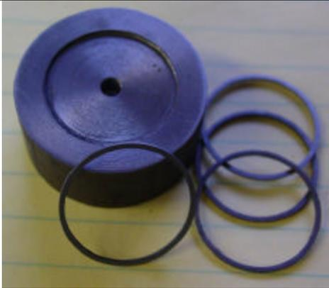
Ring Holder for sanding to thickness
