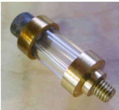
One drop every 10 minutes seems ideal and leaves an oil film on the valves and top of the cylinder. Cylinder oil is critical when using fuels that do not contain oil.
