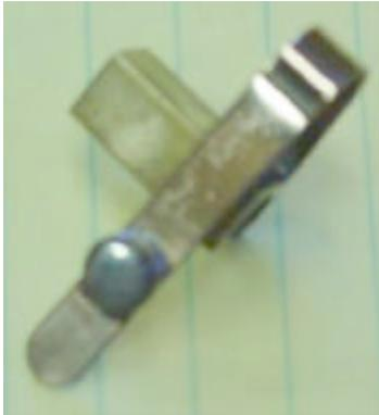
One finger is a beryllium copper spring that is moved by the cam follower. Thin spring steel could be used if the beryllium copper is not available. A bending jig is made by putting a 3/8 dowel in a block of wood, and then clamping a second piece of wood to hold the short tail as the J shape is formed. This finger is soldered to the brass grounding block.
